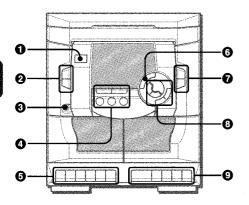
**1 POWER OSTANDBY/ON**Switches the unit on and off (standby).
